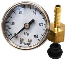
The TufGauge is installed on the supply line and allows the installer to ensure the system is running at an appropriate pressure (under 100 kPa for bottom feed systems). It is also a useful tool in troubleshooting any potential issues with the system down the track.
